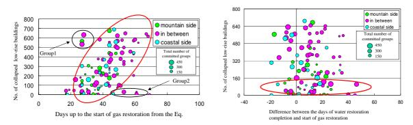
Figure 5 Effects of the damaged buildings on the recovery activities of gas system
