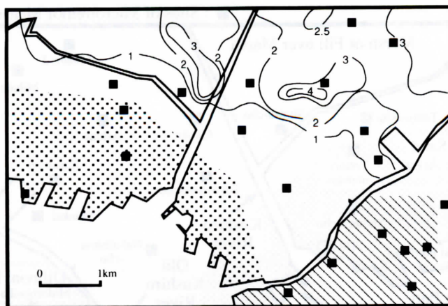
Figure 4. Contour map on the thickness of a peat layer
