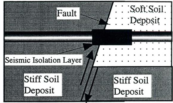
(b) Section near fault or fracture zones
