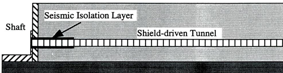
Fig.5 Schematic diagram to demonstrate the application of seismic isolation to a junction with a shaft
