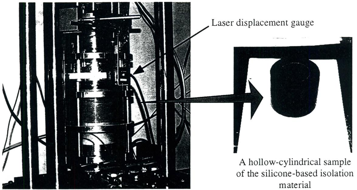
Photo.1 Dynamic shear test using a hollow-cylindrical cyclic shear apparatus
