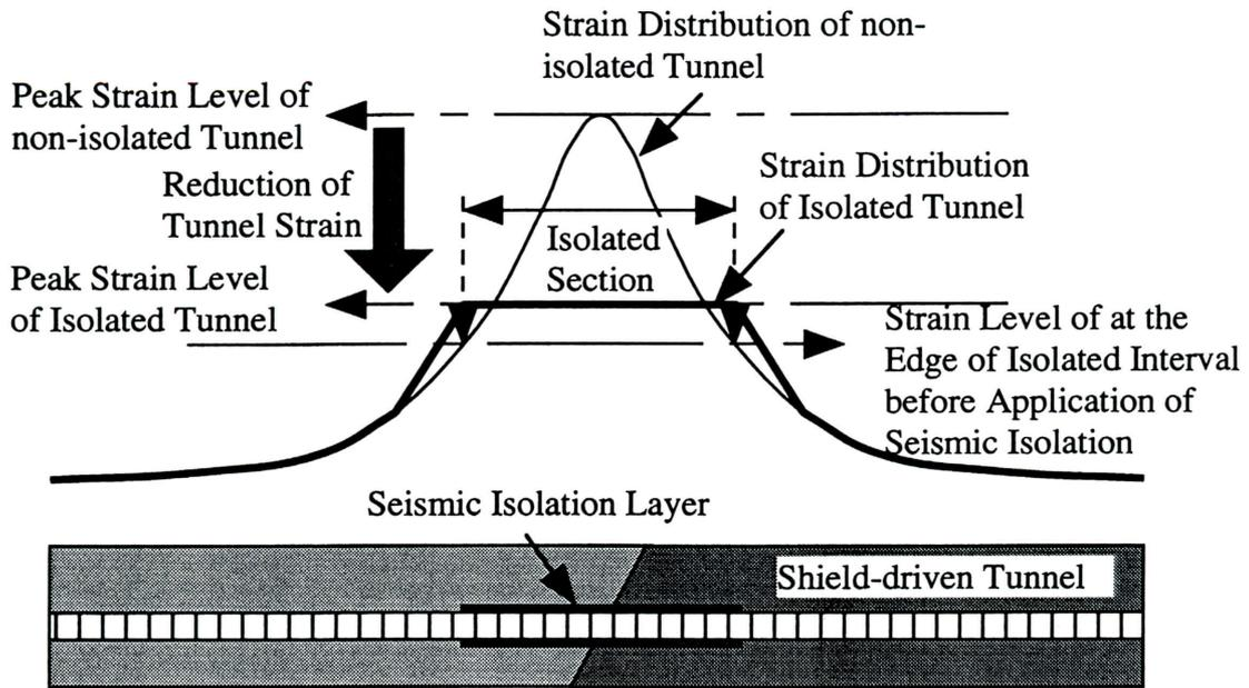
Fig.4 Schematic diagram to demonstrate the application of seismic isolation to the boundary between soft and stiff soil deposits
