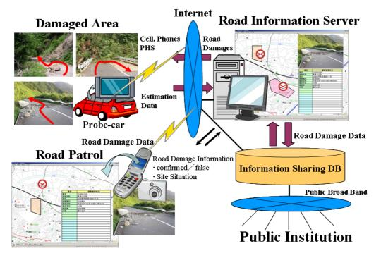
Figure 1: Schematic representation of the proposed road damage information system.
