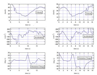
Figure 5. Time histories of driving data in case of opposite lane driving by passing
