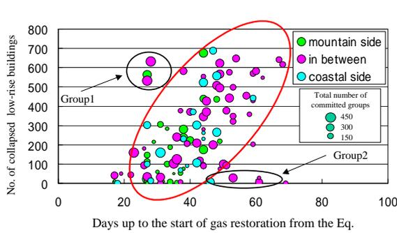
**Figure 5 Effects of the damaged buildings on the recovery activities of gas system**
