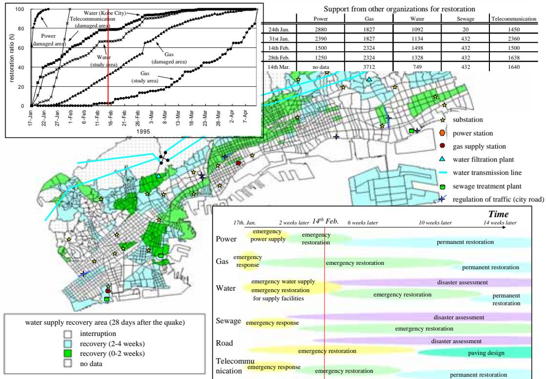
Figure 3 Water recovery area (28 days after the earthquake)
